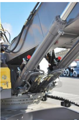
Soft swing system and BSS Boom Suspension System for higher comfort
