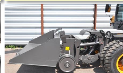
Rail cassette with bucket
