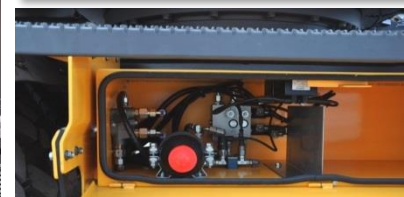
Trailer brake, operated by brake pedal
