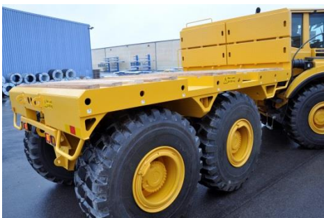
Holes for lashing chains
